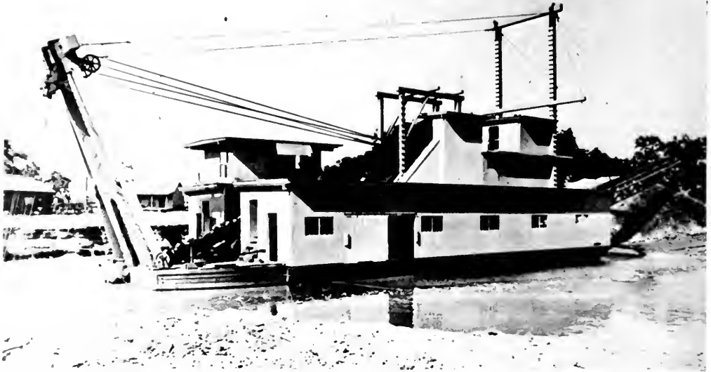
Photo 53. Cherokee Mining Company Dredge, Oroville District. This 1904 photo shows one of the earliest bucket-line dredges in California, operating here in Butte County.
