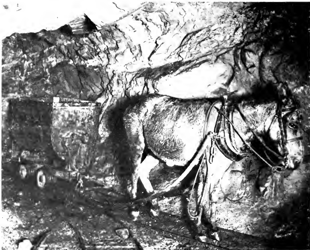
Photo 22. Empire Mine, Grass Valley District. Mules frequently hauled ore cars, as in this underground scene at the mine in Nevada County. The photo was taken in about 1910.
